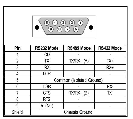
Figure 10: DB9 Port pin-out
